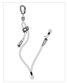
• Remove the connectors from the individual strands. Remove the protective sleeve from the lanyard side, and the rope clamp, in order to check the hidden areas.
