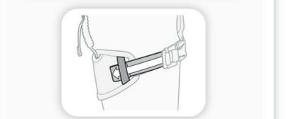
6. EN 358: 2018 harness for work positioning and restraint
